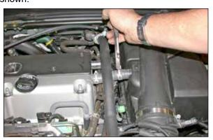
3. Using a pair of pliers, depress the hose clamp and slide it back off of the crank case vent on the air cleaner assembly as shown.
