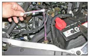
12. Using a 10mm socket, loosen the bolt that secures the air inlet duct as shown.
