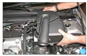
8. Loosen the 5 bolts and pull upwards to remove the upper air cleaner assembly as shown.
