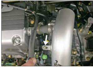
20. Using a 10mm socket secure the bracket to the air cleaner mounting point using the provided bardware.
