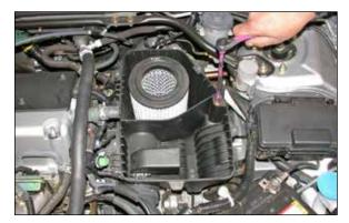
10. Loosen and remove the two bolts and one nut on the lower air cleaner assembly as shown.
